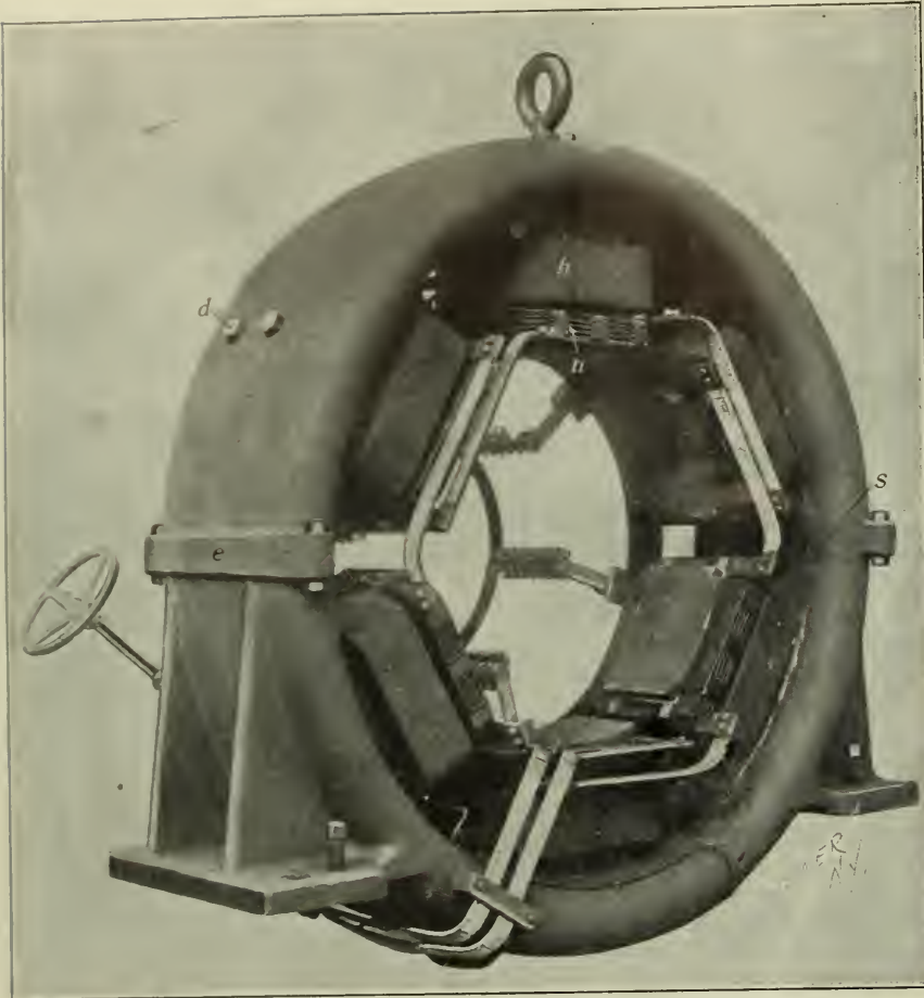
FIG. 295. FIELD FOR WESTINGHOUSE ENGINE-TYPE GENERATOR, WITH HORIZONTALLY SPLIT FRAME
